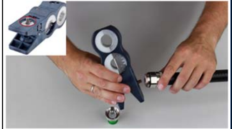
12) Start in expanded point and flare outer conductor with flaring tool by turning.
