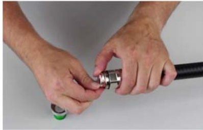
10) Put clamp ring onto outer conductor
