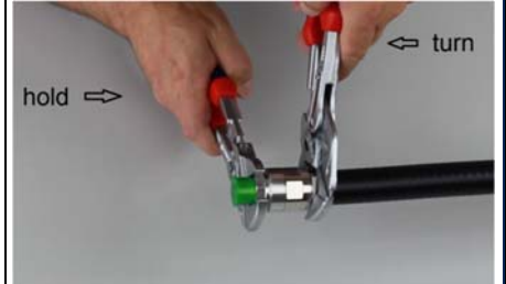
18) Tighten sealing nut with wrenches (Recommended torque: 18Nm)
