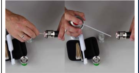
15) Clean the inner conductor with alcohol, cleaning sticks and compressed air.
