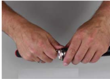
11) Expanding outer conductor on one point with a screwdriver
