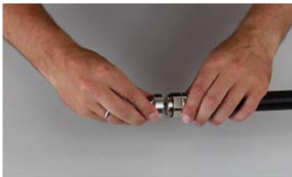
16) Put connector head by hand onto the cable and fix it with the back nut by hand. Attention: Only turn the back nut, not the connector head.
