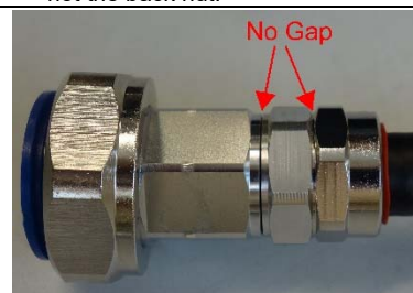
18) Put connector head by hand onto the cable and fix it with the back nut by hand. Only turn the connector head, not the back nut.
