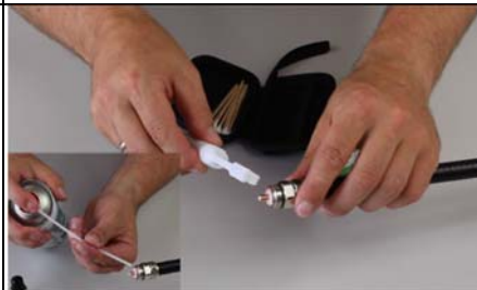
17) Clean up the cable end with brush, alcohol and compressed air.
