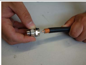
13) Please loose sealing nut slightly (not complete) in order to easily install the back nut.
