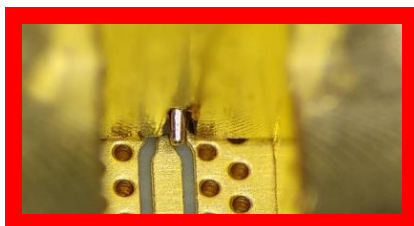
Figure 5: Detail - bad positioning
