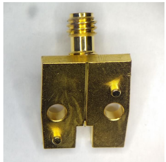
Figure 3: PCB side of solderless connector with dowel pins
