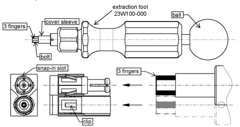
Insert the extraction tool (23W100-000) till it pushes up the housing (the cover sleeve and the bolt with the ball are pushed back simultaneously)
