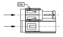
Push the connector into the housing in such a way that the clip engages noticeably into the snap-in slot
