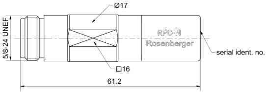
All dimensions are in mm; tolerances according to ISO 2768 m-H
